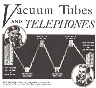
You know that the vacuum tubes in your radio set amplify the sound waves picked up by the aerial-that the more tubes the set has the greater the distance range and volume output. But did you know that vacuum tubes are also used by the telephone so that a voice may be heard as clearly over a 3000-mile circuit as it is over one of 3 miles?
